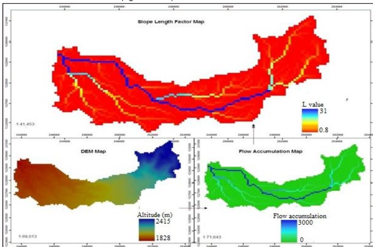
Figure 4: Derivation of slope length (L) factor from flow accumulation and slope data
