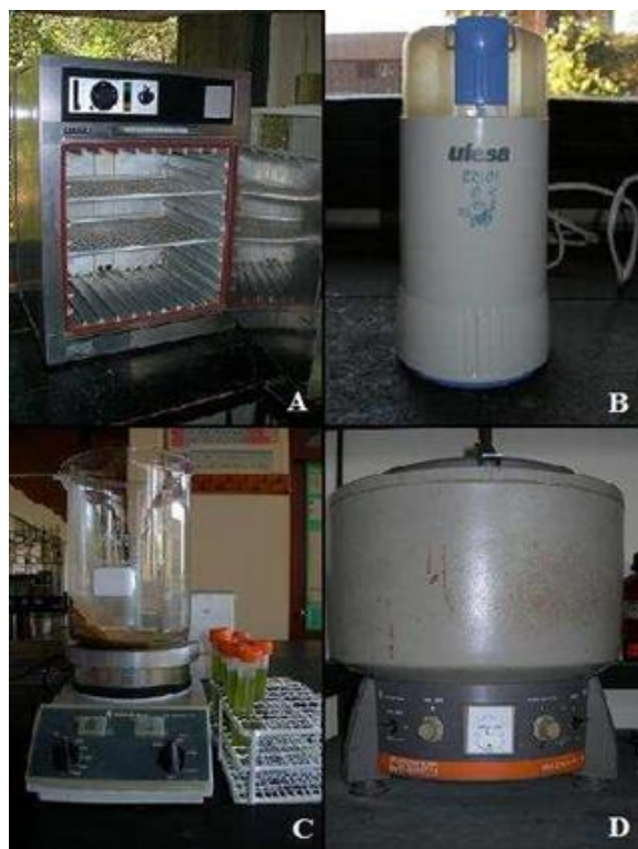
Figure 2. Laboratory equipment. A) Forced air stove; B) Electric grain mill; C) Magnetic stirrer; D) Centrifuge.
